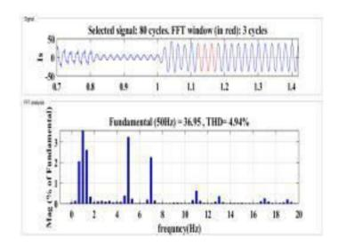
figure10.frequency spectrum of DSATCOM for RL load
