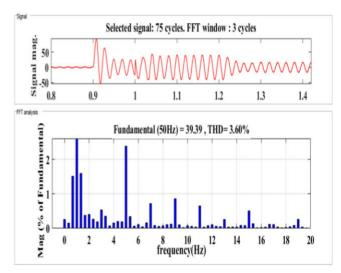
Figure6 frequency spectrum of DSTATCOM for dynamic load
