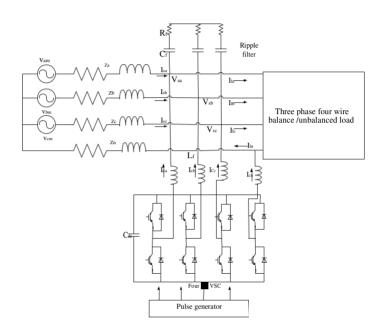
Figure 1. Schematic diagram of four leg VSC of DTATCOM connected to three phase four wire system
